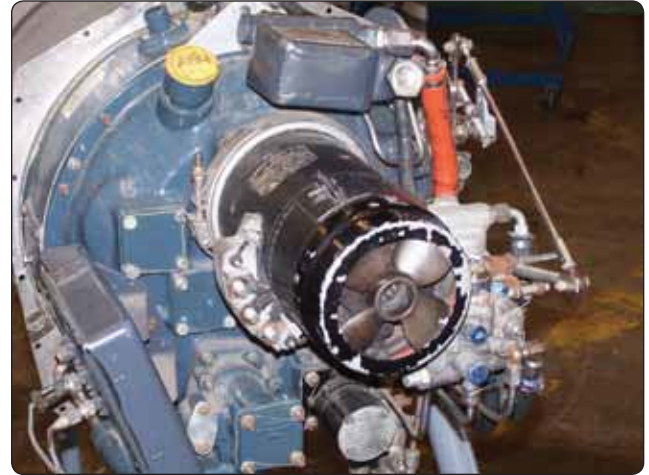
Figure 1-45. Typical turboprop accessory case.
