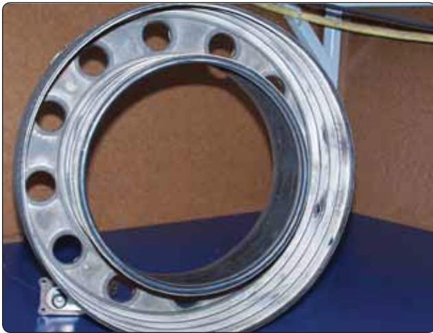
Figure 1-58. Annular combustion with chamber ceramic coating.
