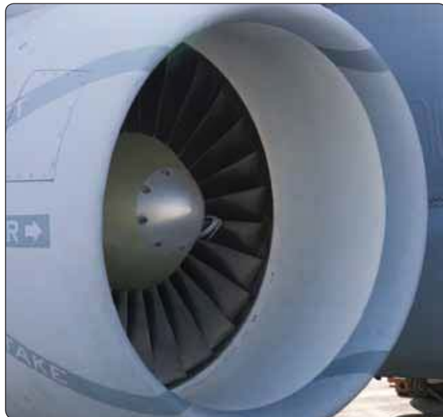
Figure 1-44. Typical turbofan inlet.
