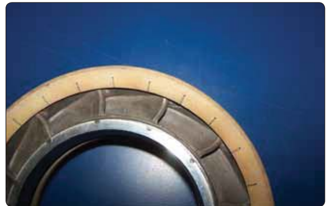
Figure 1-60. Turbine inlet guide vanes.
