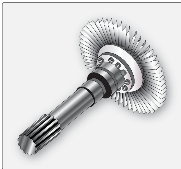
Figure 1-63. Rotor elements of the turbine assembly.
