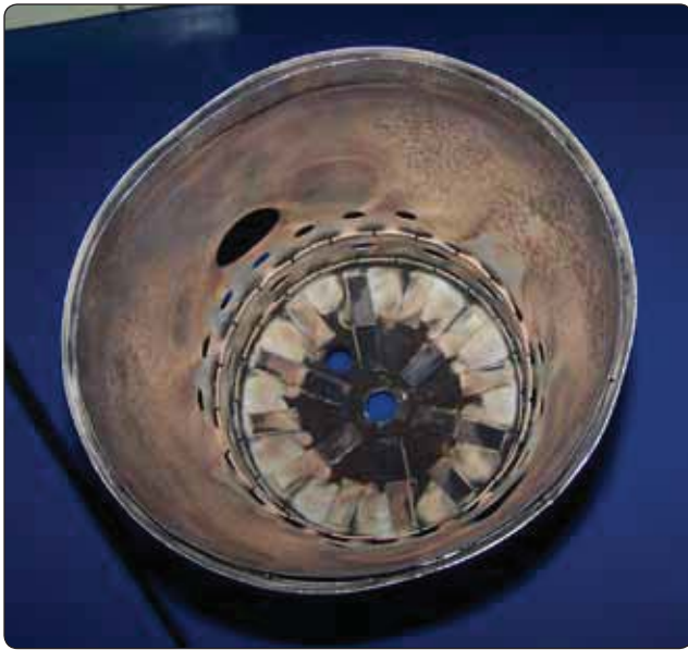
Figure 1-53. Inside view of a combustion chamber liner.
