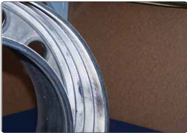
Figure 1-55. Annular combustion chamber liner.
