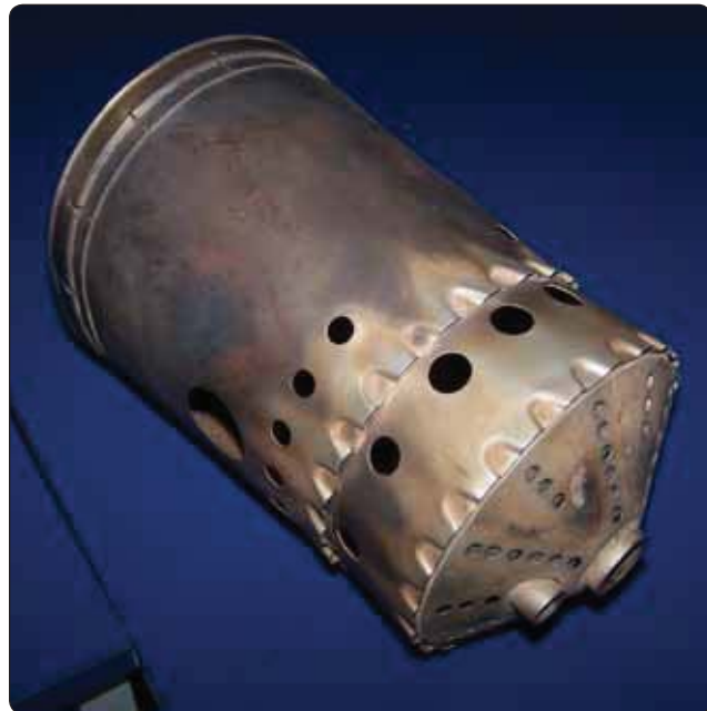
Figure 1-52. Can-type combustion chamber.
